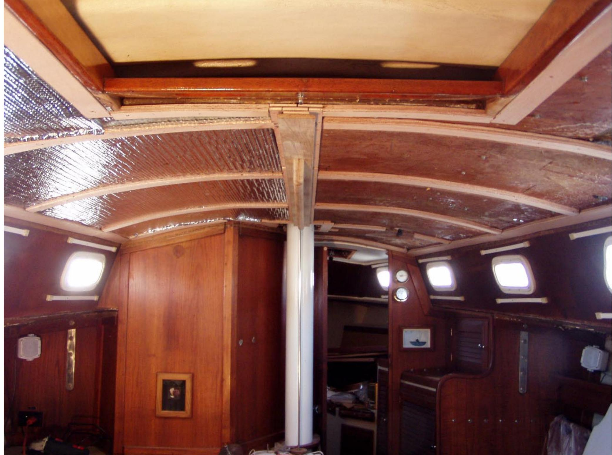
Insulation has been glued between firing strips
