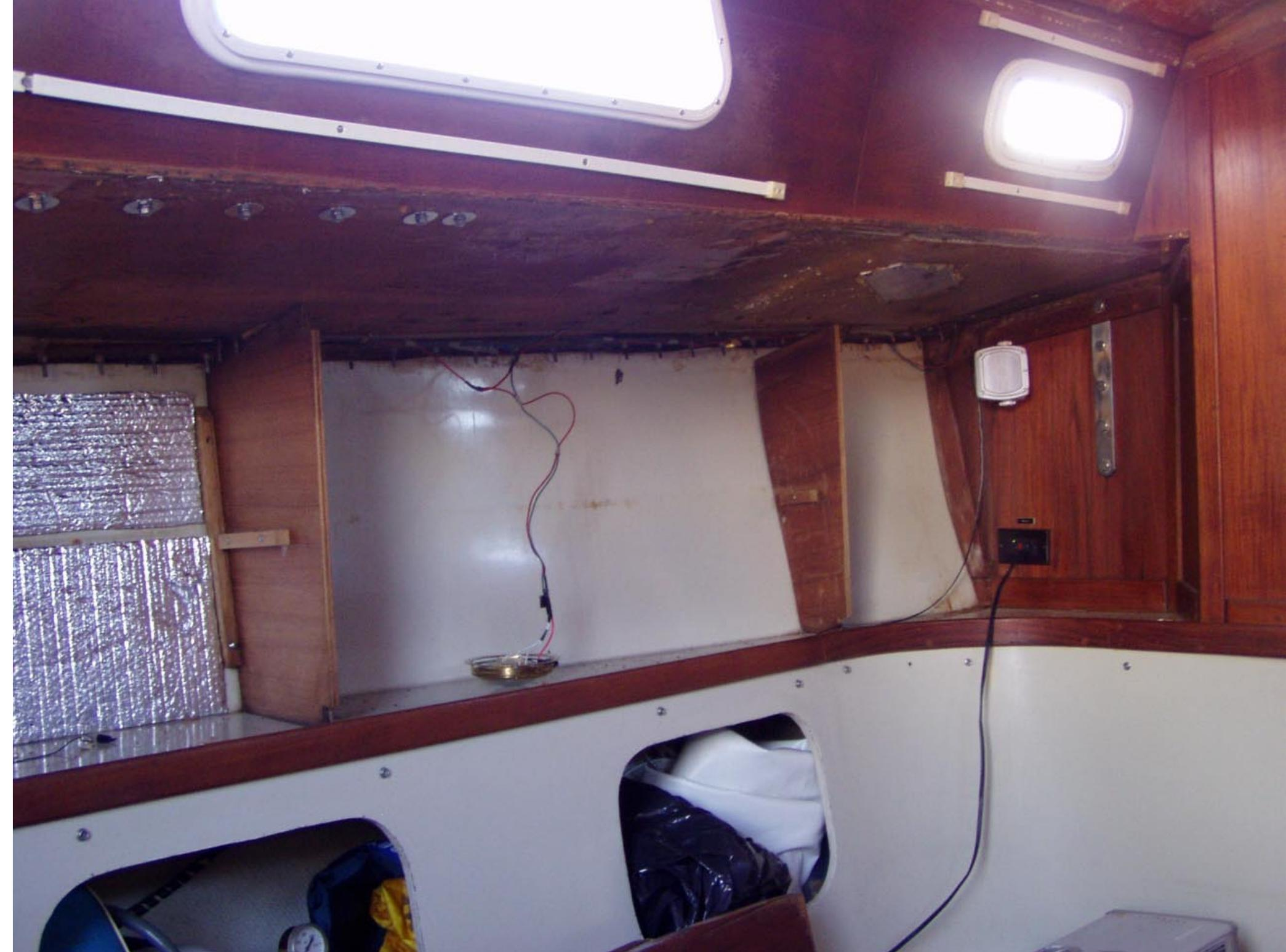
Port side cabinetry removed in order to insulate hull, deck and coach top
