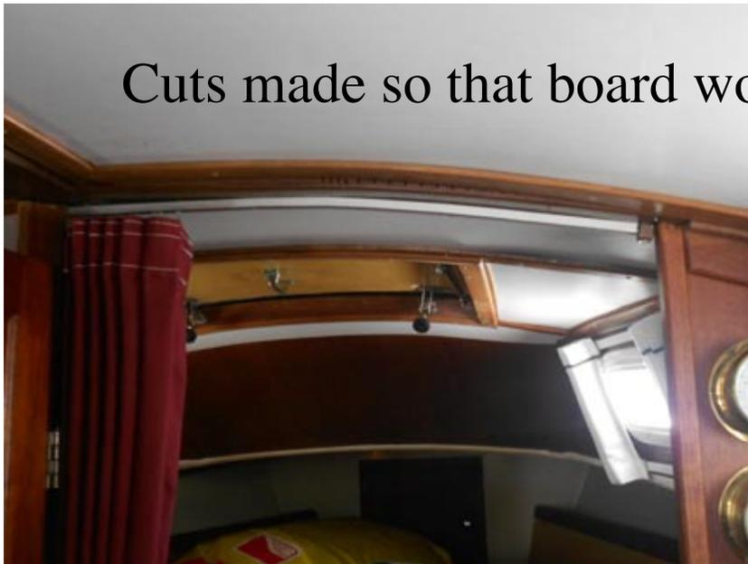
Cuts made so that board would bend to curve of cabin top
