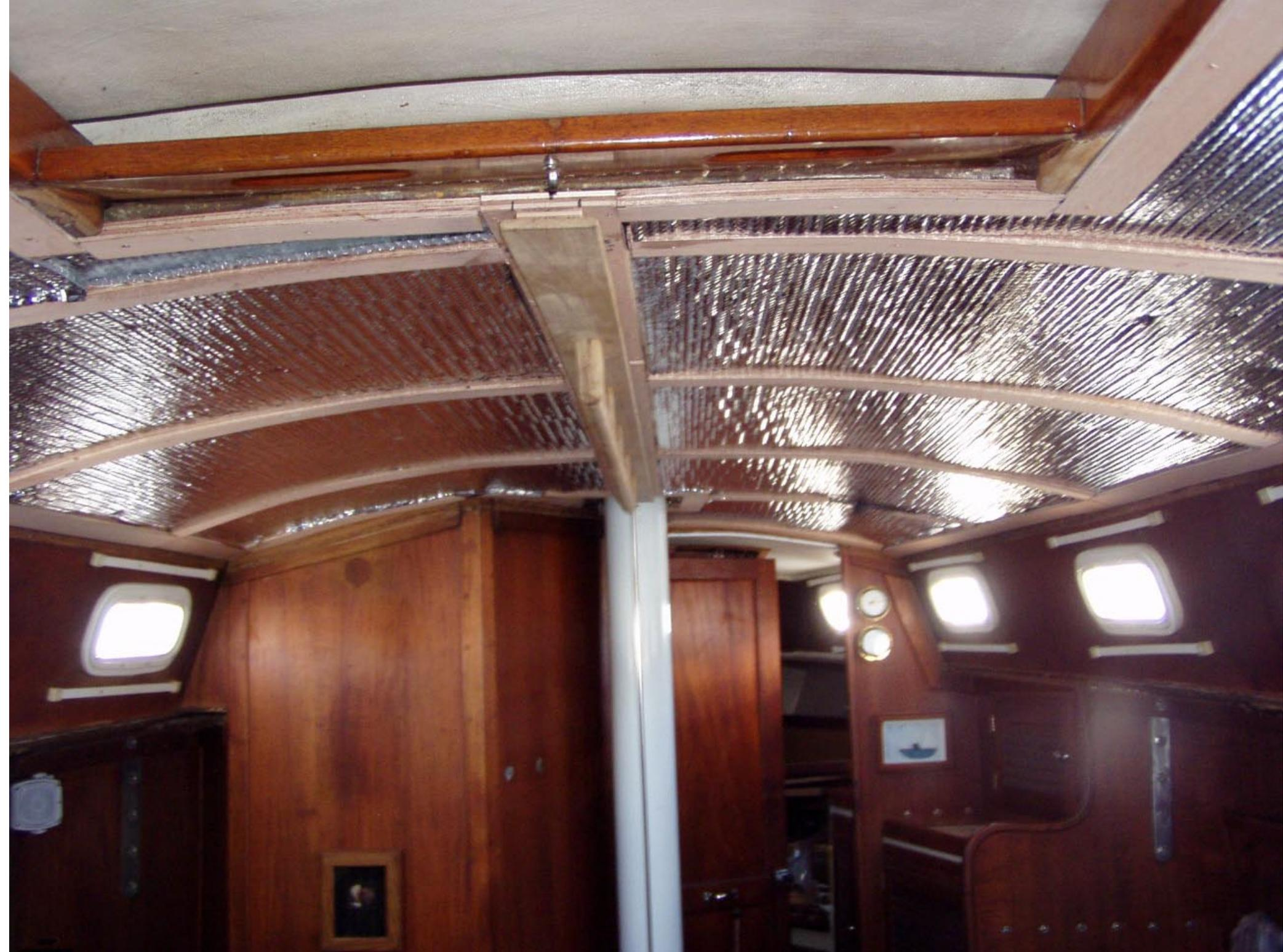
Insulation has been glued between firing strips
