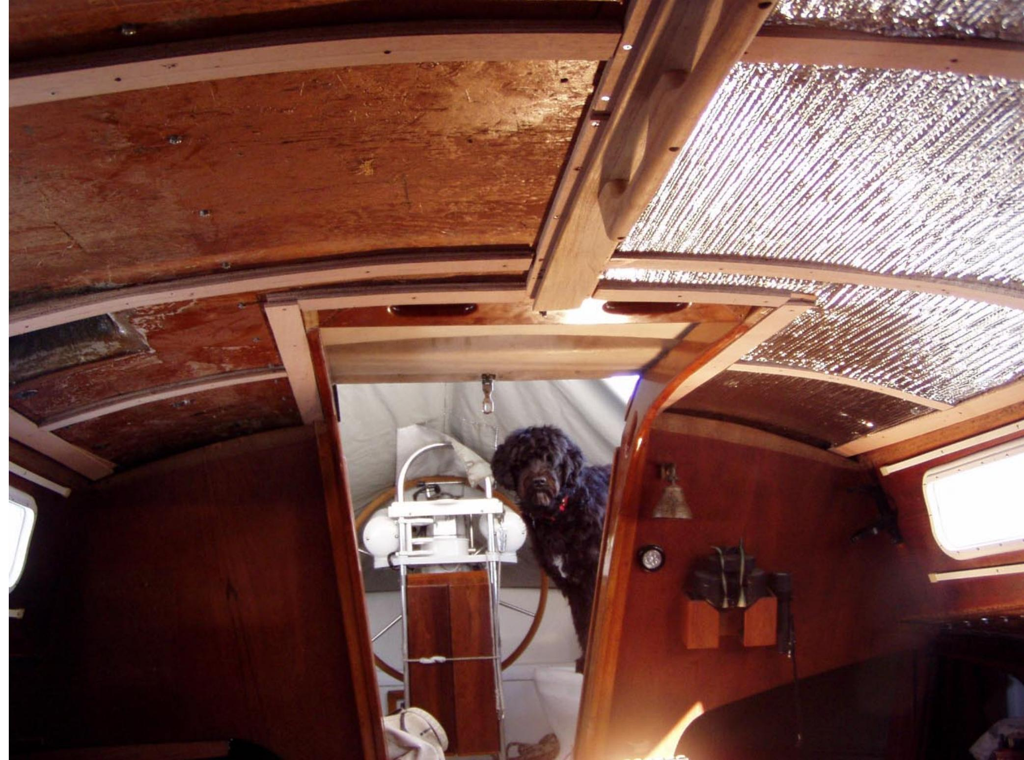
Insulation has been glued between firing strips
