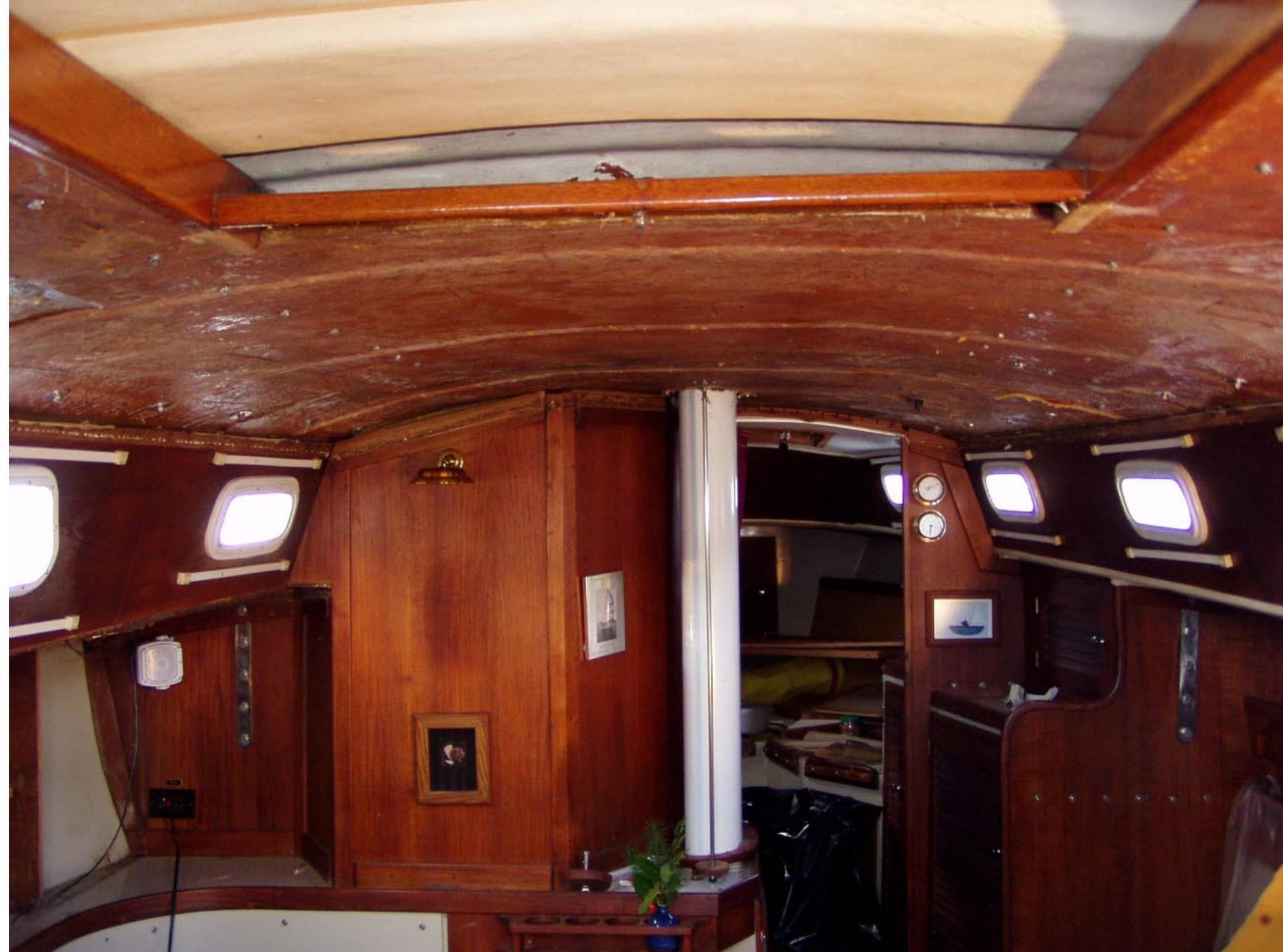
Headliner and foam backing has been removed
